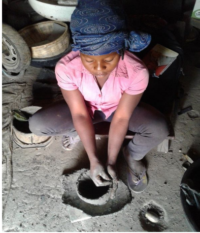
Plate 1a: Molding the pot
