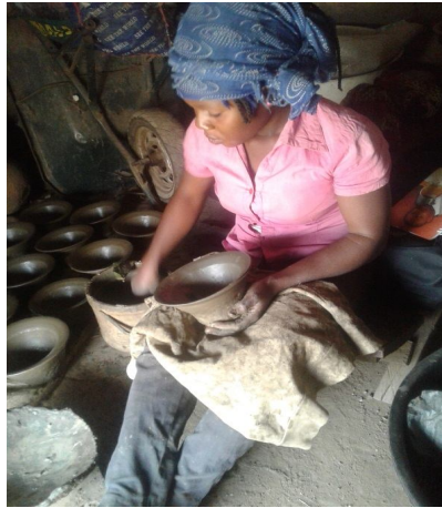
b: Forming the rim on the pot
